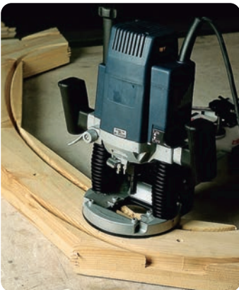
Uses standard electric router
