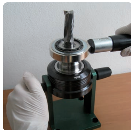
Tighten the nut using the torque wrench Art Z052 page 10.08
