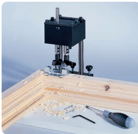
Fixing of top hinge
