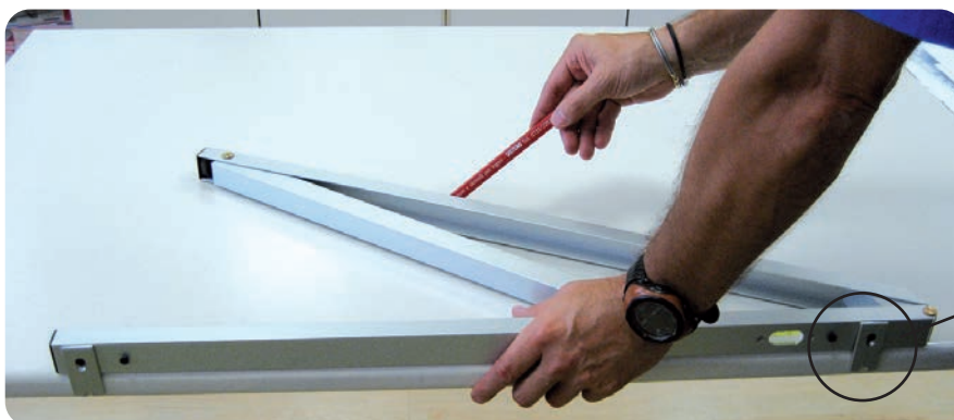
Angolfast 70S with reference shoulder for easier outlining.
