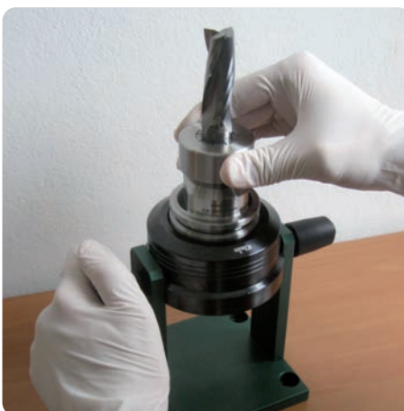
Insert the collet chuck in the demount devices
